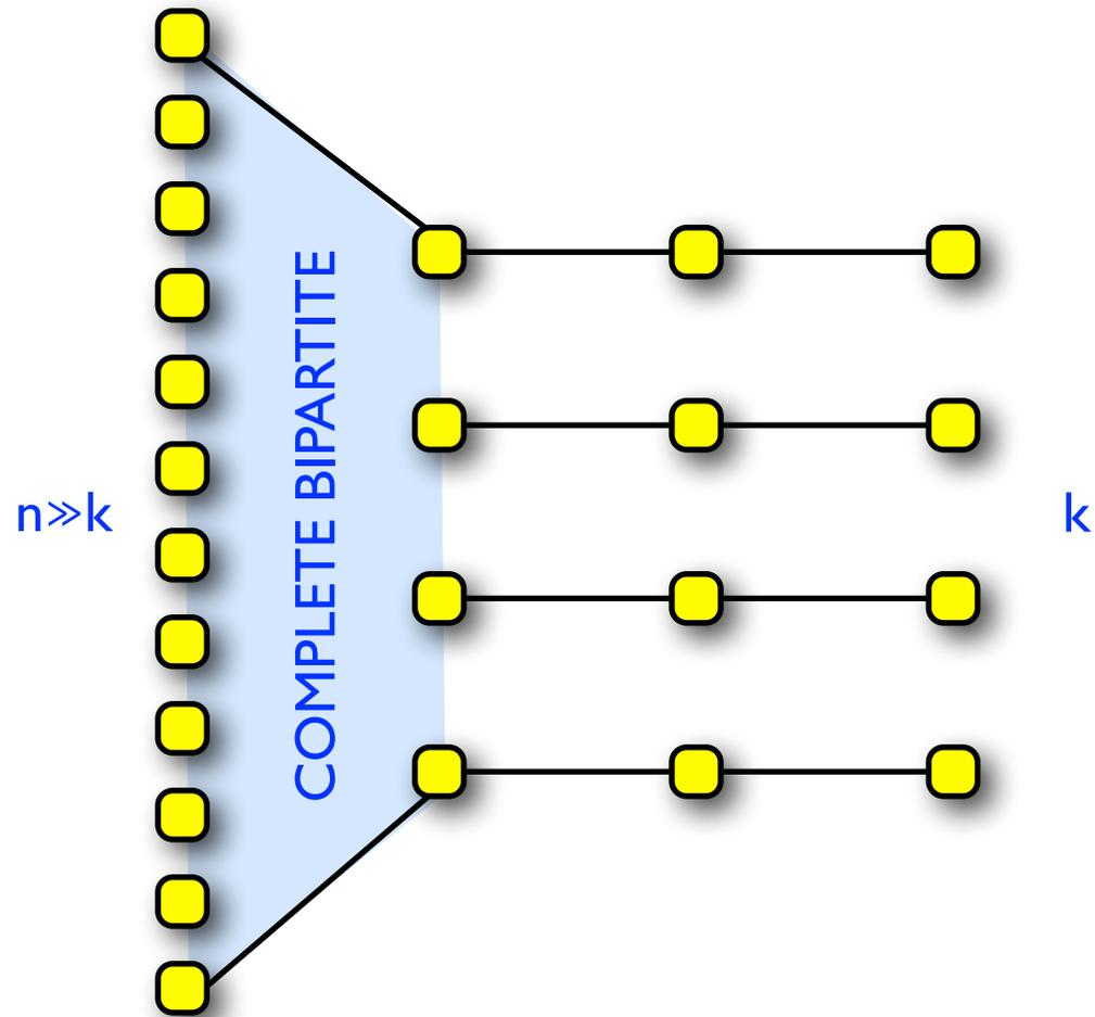
Need to uniformly sample  $\Omega(kn)$  edges before we find a matching of size  $2k$ .
